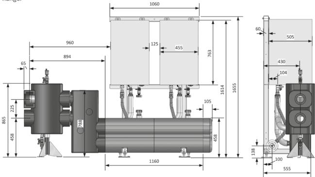
The 2 boiler in-line cascade frame for Sirius two WH 90 & 110 Kw outputs have a Manifold pipework size of DN100 and the frame sizes differ from the above due to the boiler size being larger. DN100 flanged faced connections are supplied for system connection.
