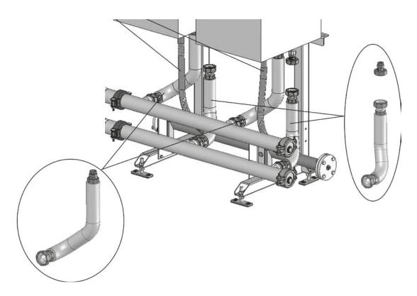
Assembling the flow connection: Please read this section in conjunction with page 18 & 19 for exploded view drawings of the connection sets.
