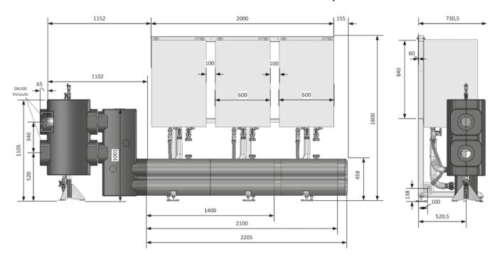
Wall Hung Condensing Boilers
