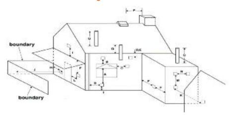
Minimum clearances for concentric room sealed flue terminals are shown below (for conventional flue systems please refer to the relevant British Standards). The terminal shall be positioned so it will not cause a hazard to health of persons who may be nearby or a nuisance to other persons beyond the property's boundary.
